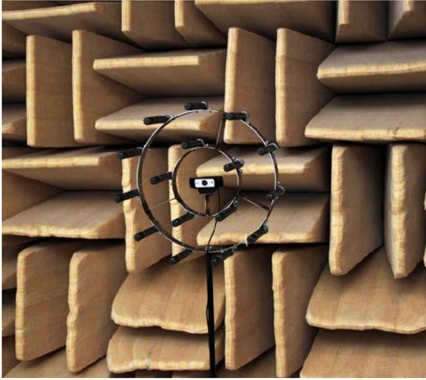
Figure 1: Developed double ring array
