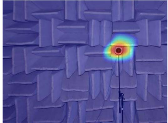
Figure 3: Resulting output image of an acoustic camera
